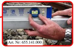
Measure the inclination of the track with a spirit level.
