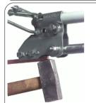
The ends of the contact wire should be bent upwards by using a hammer.
