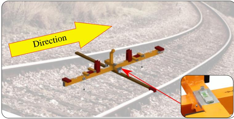
Place the JIG in a user-defined installation position. Adjust the level gauge.
