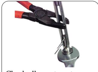
Check all counter nuts once more. Block turnbuckles with counter nuts.
