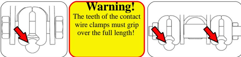
Tighten the bolts of the contact wire clamp with **50 N m** by using a torque wrench and **retighten 2 times** (until each bolt has been tightened 3 times).
