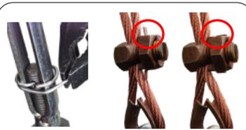
Lock turnbuckles with a locking wire. Fix the locking device.
