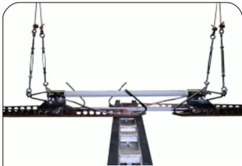
Check with spirit level or pantograph for optimal gliding.
