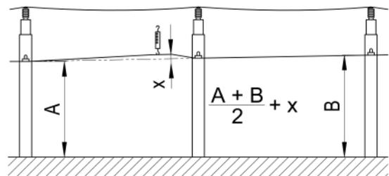
When replacing an existing section insulator measure the height of the contact wire at masts A and B. Calculate the average value. The hogging value should be minimum  $x = 70$  mm.
