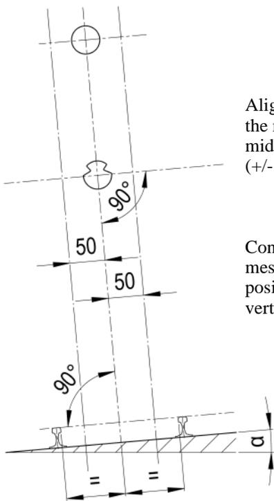
Align the contact wire and the messenger wire in the middle of the track (+/- 50 mm).
