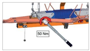
Tighten the nuts to **50 Nm** and lock them with the second nut.
