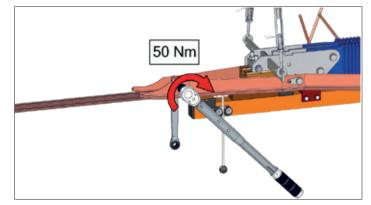
Remove the installation JIG from the insulator body.
